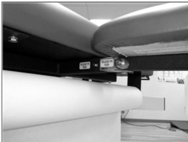
Figure 10. Place a role of paper on the paper dispenser rod and install the rod between the brackets. Press in on either spring-loaded end of the paper dispenser bar in order to slide it into the brackets.
