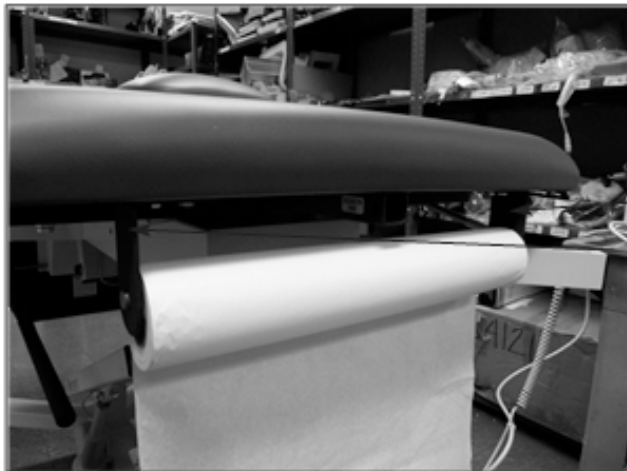
Figure 9. Using a 7/16" wrench, install the two 1/4-20" hex head screws removed in step 1 through the dispenser mounting bracket and tighten to secure the paper dispenser bracket in place. Repeat steps 1 - 4 for the opposite side.
